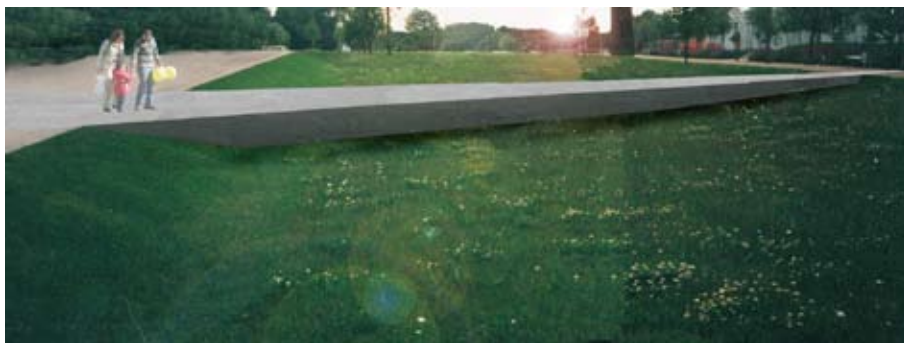
The sports fields and other areas will be sunken to allow flooding during major storm events
